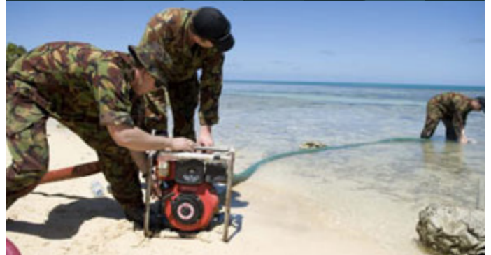
NZ Defence Force soldiers pump salt water into a reservoir for desalination. Credit: New Zealand Defence Force
